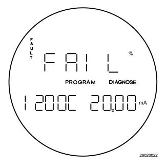
Figure 6-3. Faulted Operation Display
